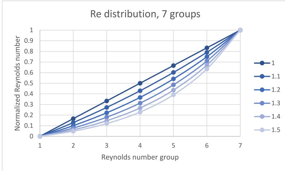
Figure 2: Normalized Reynolds number (0-1) for seven Reynolds number groups, with adjusted bias factors. A bias factor of 1.0 indicates even distribution of Reynolds numbers, while increasing this factor biases more test points near the lowest Re.
