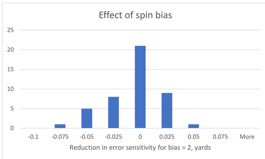
Figure 6: The reduction in the error sensitivity of all setting based on setting intermediate spin values 1/3 of the span between the minimum and maximum values (bias factor = 2) rather than midway (bias factor = 1).
