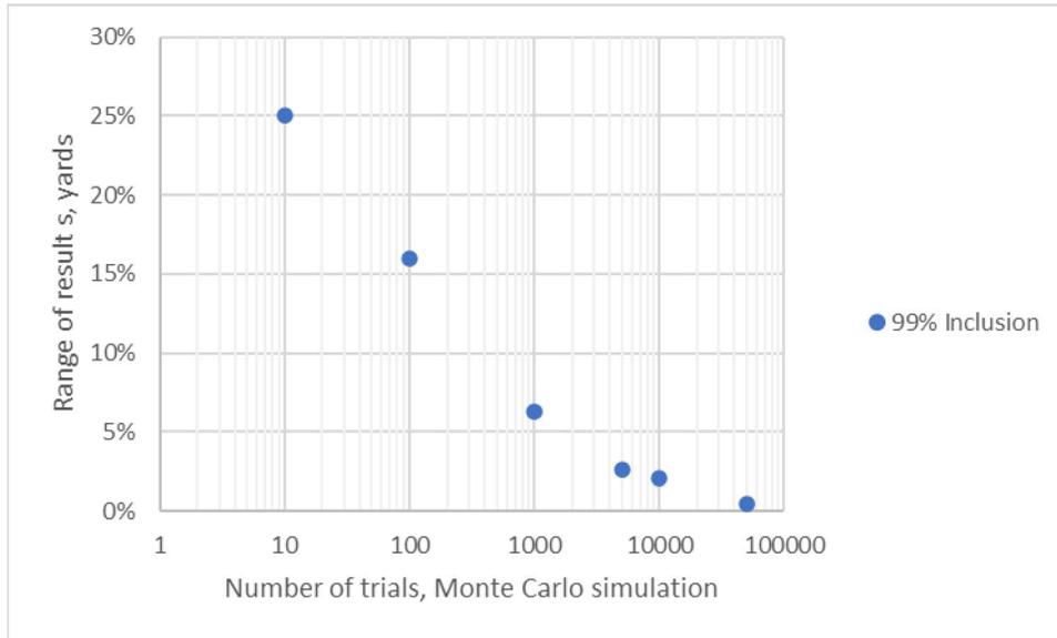
Figure 3: Range of uncertainty in estimate of the standard deviation of overall distance resulting from random error, as a function of the number of trials in Monte Carlo simulation.
