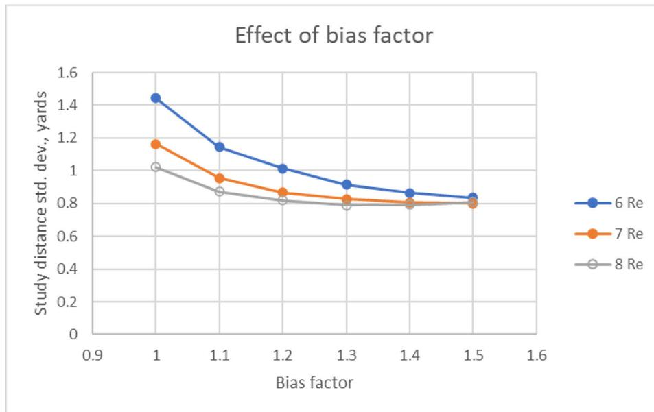
Figure 4: The effects of increasing the Reynolds number bias factor. Examples where two spins at each Reynolds number were evaluated are shown (spin bias factor = 1).
