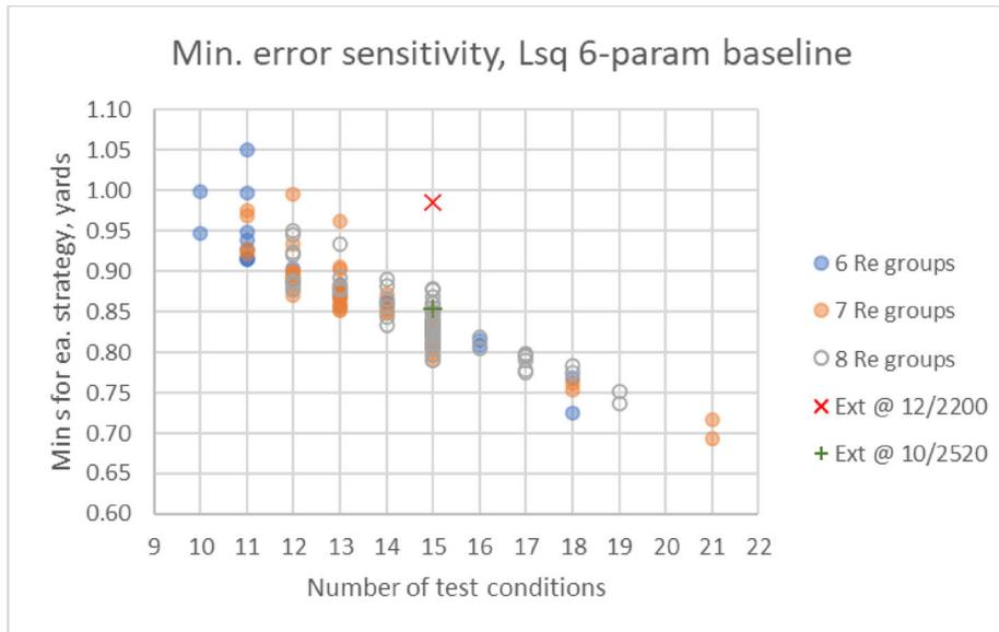
Figure 5: Minimum error sensitivity as expressed by the standard deviation of total distance estimate in response to lift and drag errors. Minima were identified through the lowest reported value based on Re bias factor (range 1.0 – 1.5).
