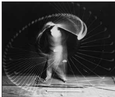
By using synchronized strobe flashes, Harold Edgerton was able to capture the swing action of Bobby Jones.
